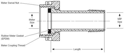
3/4" and 1" Meter coupling made of brass
